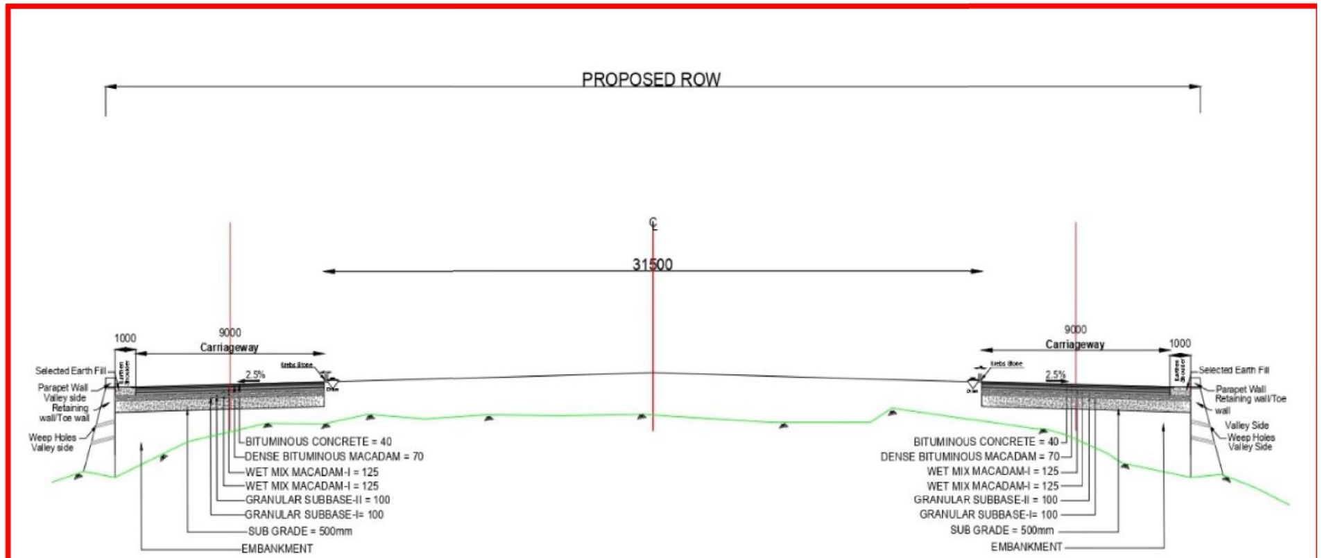
TYPE - 7 TYPICAL CROSS-SECTION FOR APPROACH OF TUNNEL WITH BOTH SIDE FILL WITH RETAINING/TOE WALL
