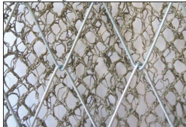
Fig. 11 – Erosion control mat
