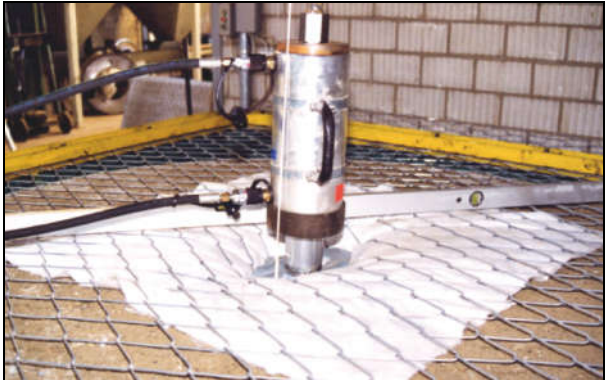
Fig. 9 – Test setup to determine the bearing resistance of the mesh against puncturing in nail direction
