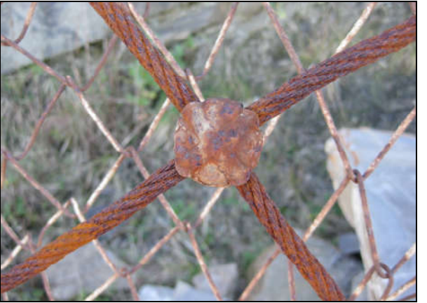
Fig. 17 – Spiral rope net corrosion protection compared to ordinary cable net system
