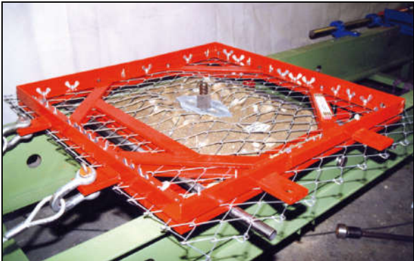
Fig. 8 – Test setup to determine the bearing resistance of the mesh against selective tensile stress parallel to the slope
