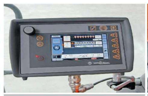
All at a glance: Important parameters are continuously displayed in the bottom menu bar of the metering menu
