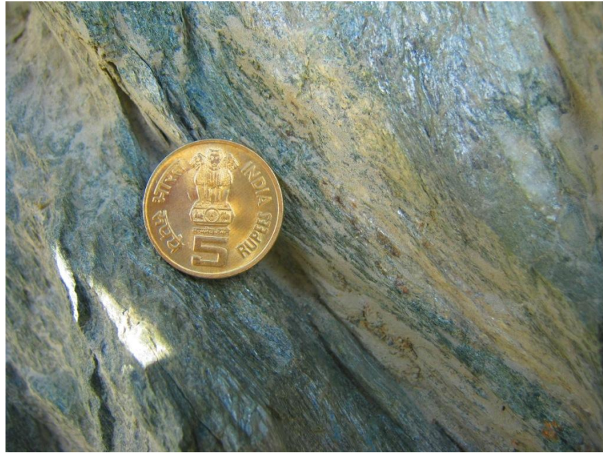
Fig. 33 A View of schistose basic rock in which Chloritic flakes are found oriented along foliation planes
