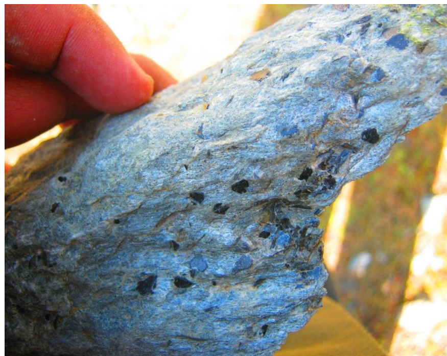
Fig. 29 A close View of Fine grained Porphyroblastic Panjal Trap rock
