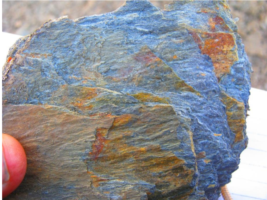
Fig .25 A Close view of Zoji-La Slates, in which fine purite cubes are noted in abundance
