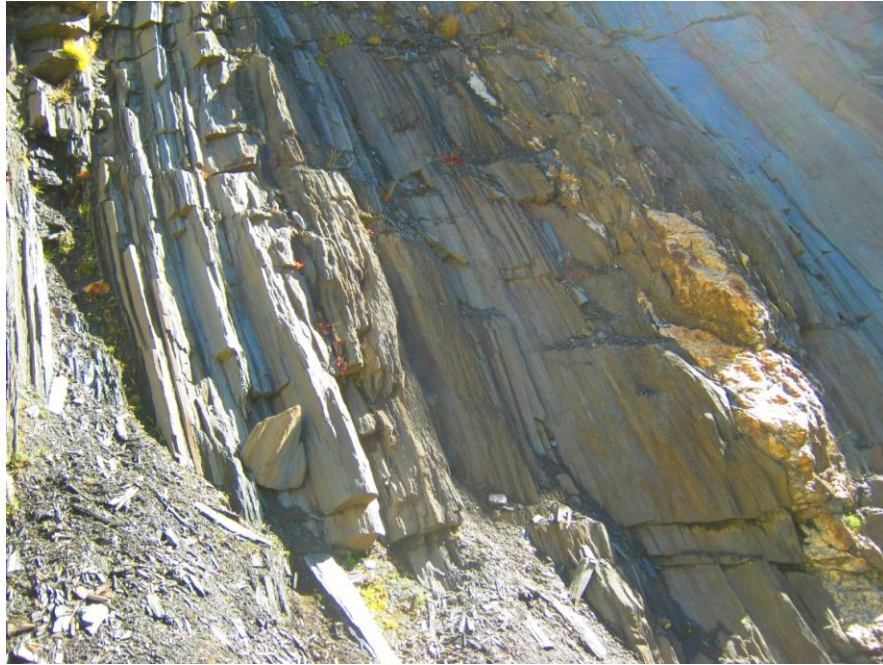
Fig. 40 A View of Three set of joints in Steep dip foliated Zoji-La formation near Zoji-La Pass
